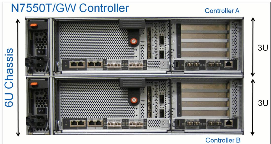
Figure 4-3 IBM N series N7550T base components
